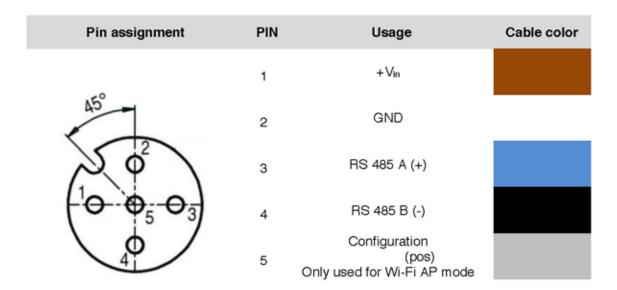
The device has a half-duplex, 2-wire RS485 interface for configuration, measured value query and firmware update.
