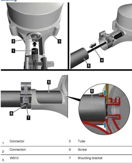
The WS10 is mounted on a tube in horizontal position. Make sure the tube is mounted safely
