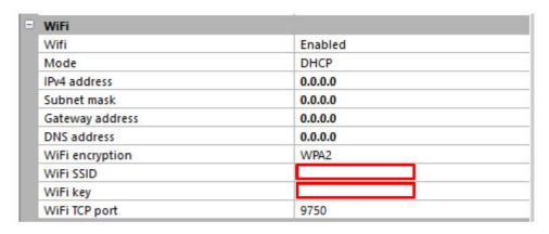
With "Save" the configuration will be written to the WS10 and the WS10 will automatically restart with the new parameters.
