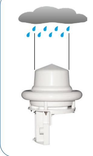
24 GHz Microwave Doppler Radar works with the radar reflection method and measures the precipitation quantity or precipitation intensity by means of the correlation of drop size and velocity.
