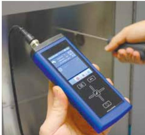
Ideal for volume measurements, air intake and air discharge measurements in climate measuring technology. Data memory, software and Manufacturer Calibration Certificate included.
