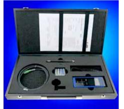
A high quality wooden case, resistiveelectrolytic sensor, 2m cable, batteries and DAkks calibration certificate are included.
